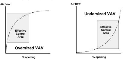
Be sure the VAV actuator is properly installed and set-up so the VAV damper blade is able to rotate from the fully opened, to fully closed position with no restriction to its mechanical rotation.
