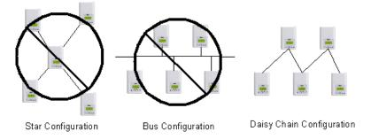
A daisy-chain wiring scheme does not allow for T connections. I.E. the network wire needs to be wired down to each thermostat communication terminals before going to the next device. No junctions of any kind are recommended to be installed. Except for the first and the last devices on the network, all thermostats should have 4 wires connected to the + and – network connection.
