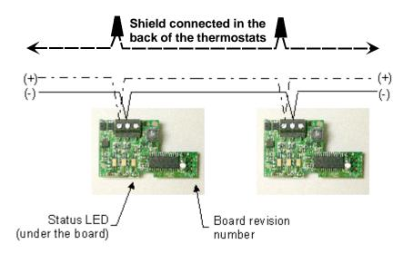
All the shield(s) attached and wired together need to be connected to the ground only at one location on the whole network.
